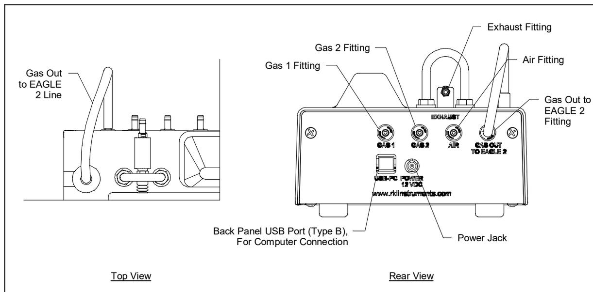
**Figure 7: Fittings and Connections**
