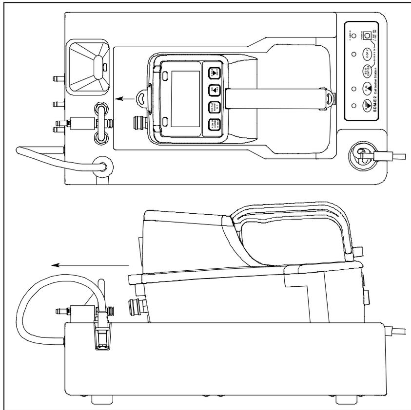
**Figure 12: Inserting the EAGLE 2**
