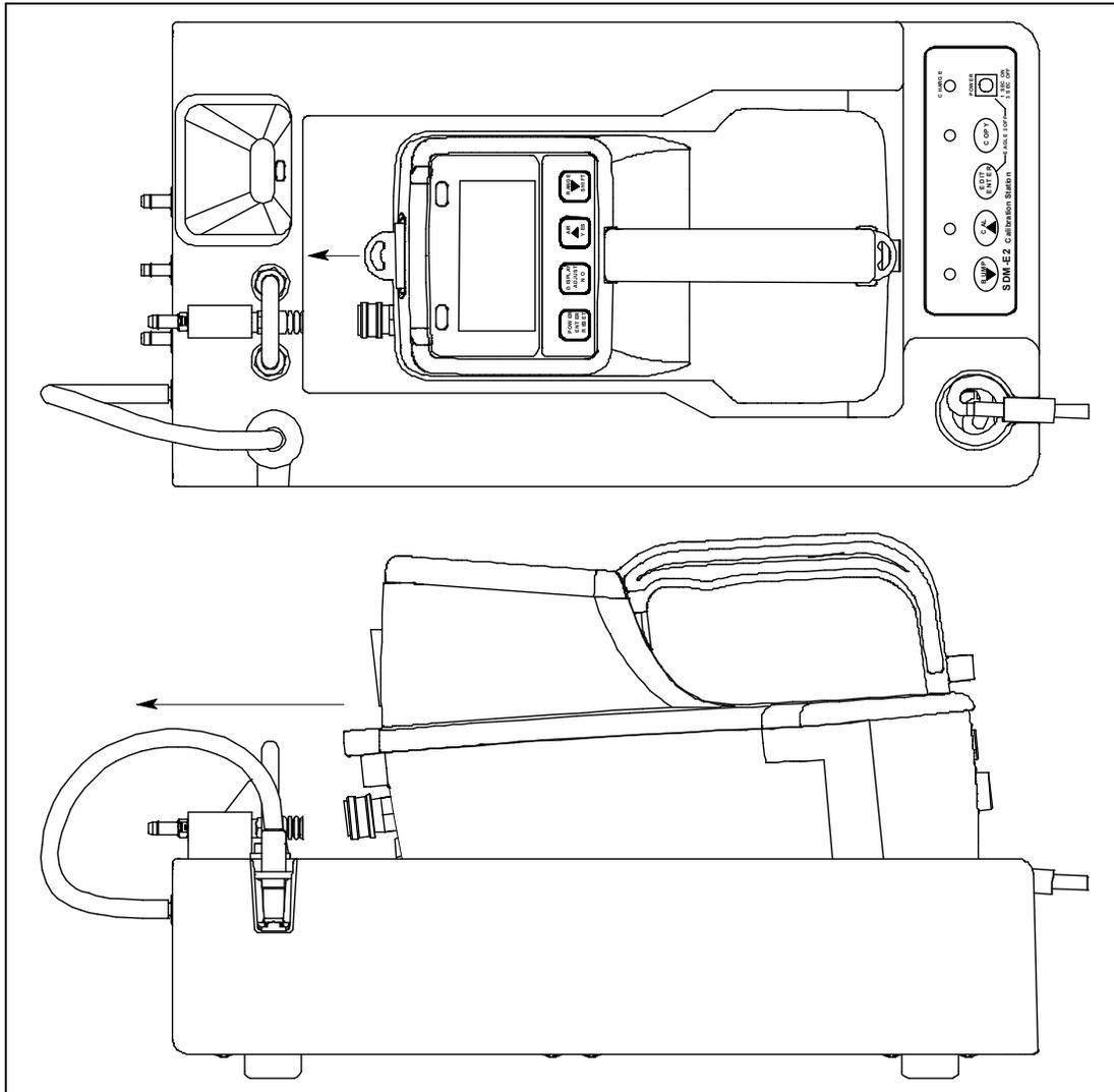
**Figure 13: Inserting the EAGLE 2**
