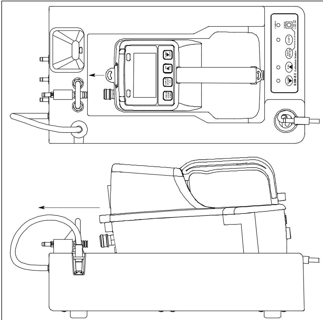
**Figure 14: Inserting the EAGLE 2**
