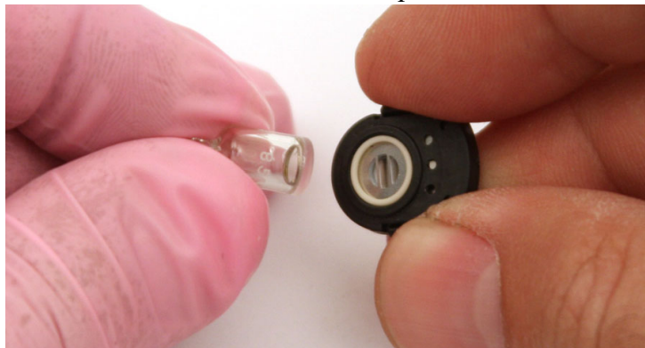
Figure 14: Reinstalling Electrode Lamp
