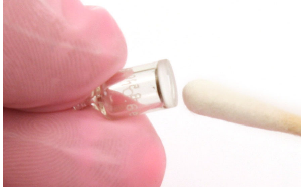
Figure 9: Polishing the Electrode Lamp Window
