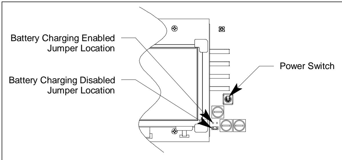
Figure 14: Battery Charging Jumper Locations
