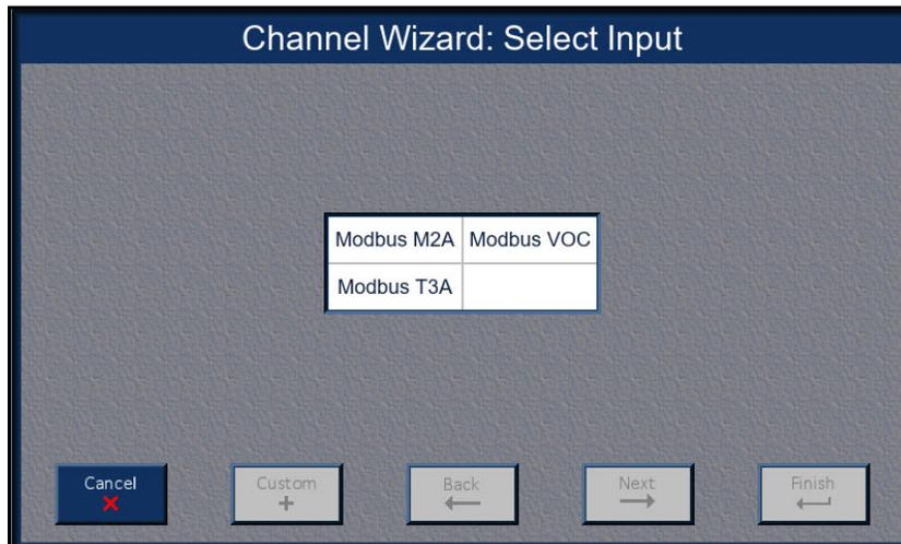
**Figure 61: Confirm Modbus Input Type Selection**
