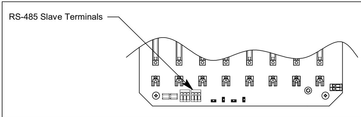
**Figure 21: Modbus Slave Terminal Locations**
