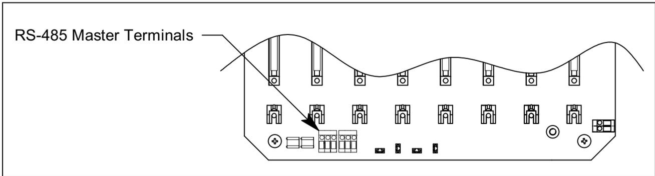
**Figure 15: Modbus Master Terminal Locations**
