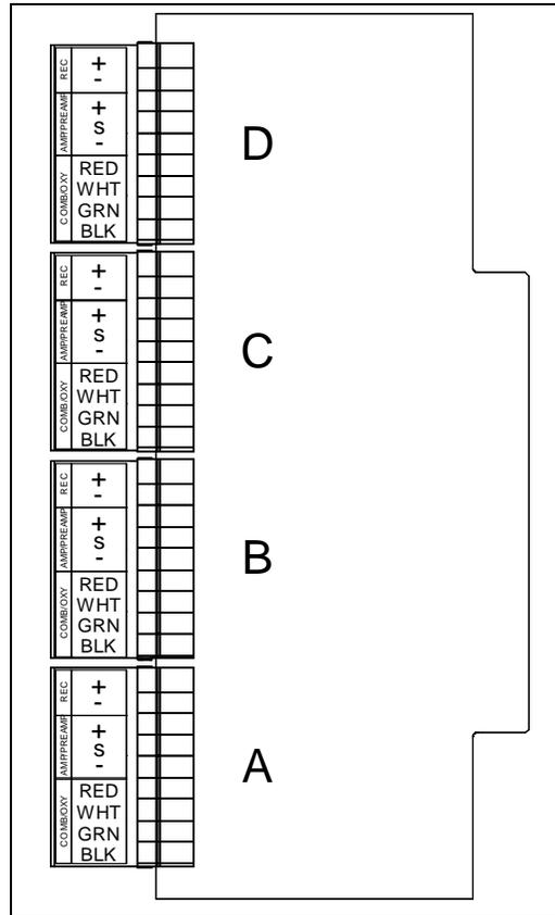
**Figure 29: Sensor Module Channel Assignment**
