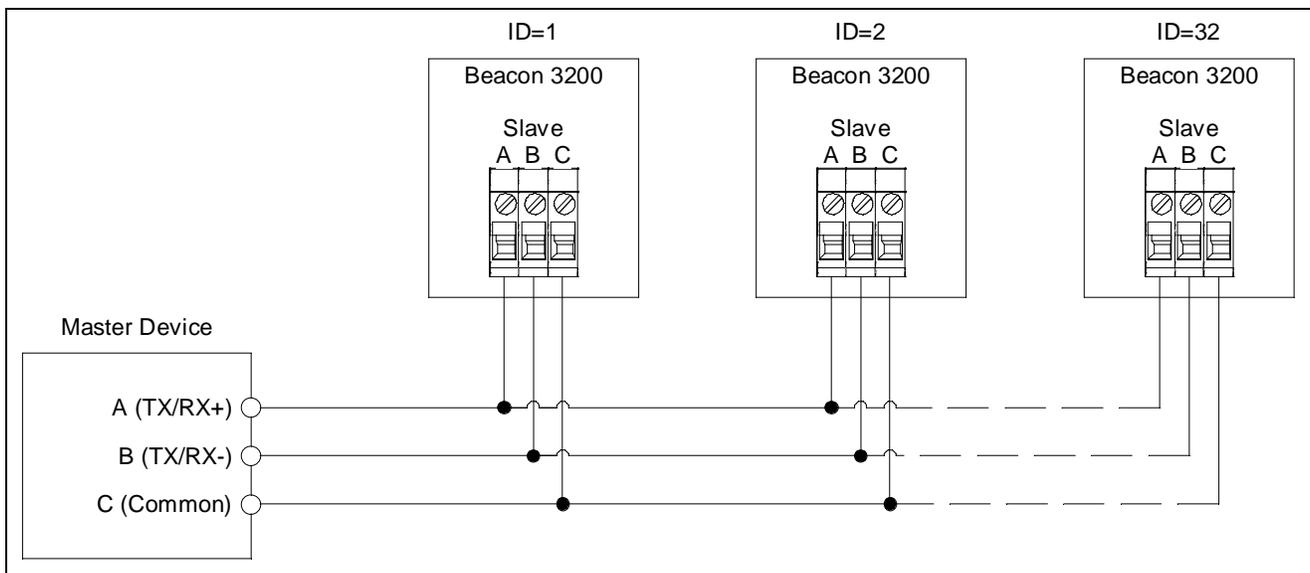
**Figure 22: Modbus Slave Wiring**
