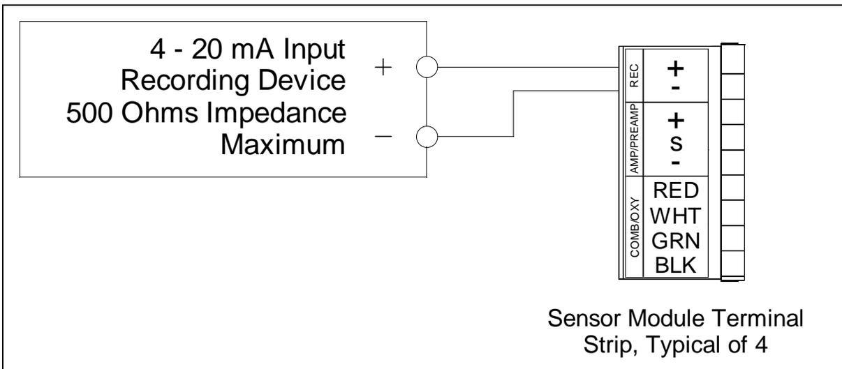
Figure 31: Recorder Output Wiring
