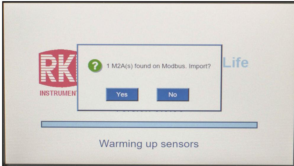
**Figure 33: Modbus Detector Discovery**
