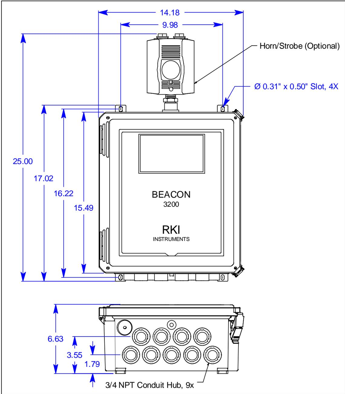
**Figure 8: Outline and Mounting Dimensions with Horn/Strobe Installed**
