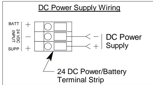
Figure 12: DC Power Supply Wiring
