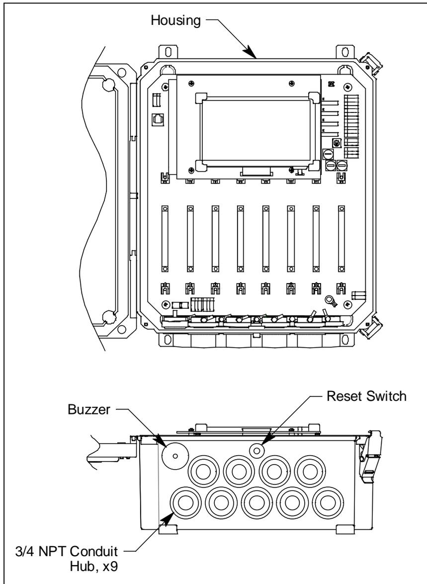
**Figure 1: External Component Location**
