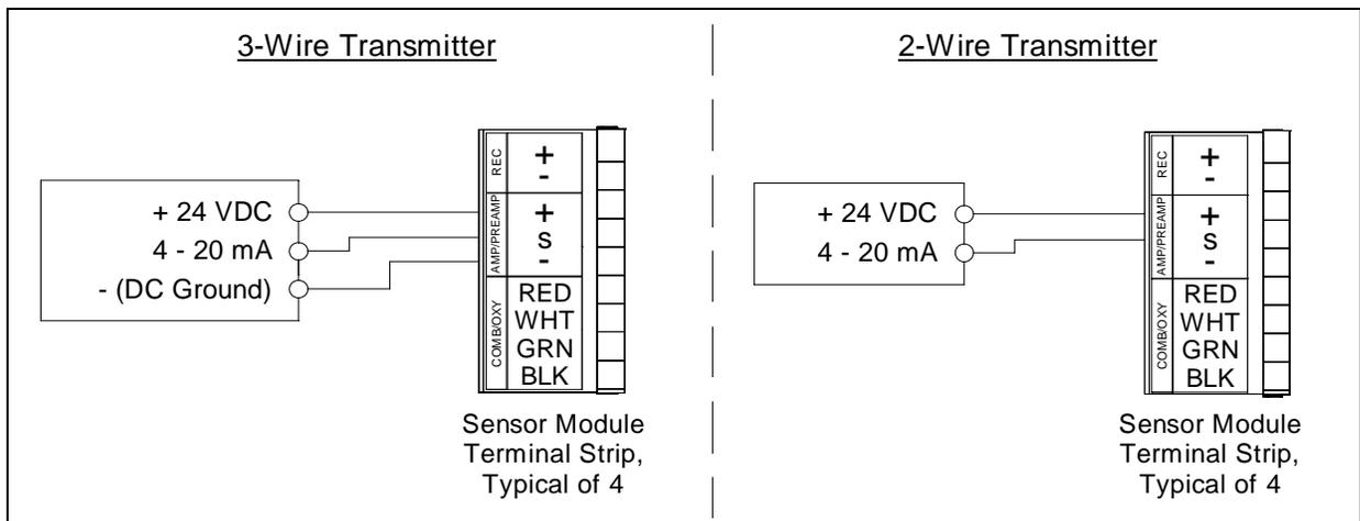
**Figure 30: 4 to 20 mA Transmitter Wiring**
