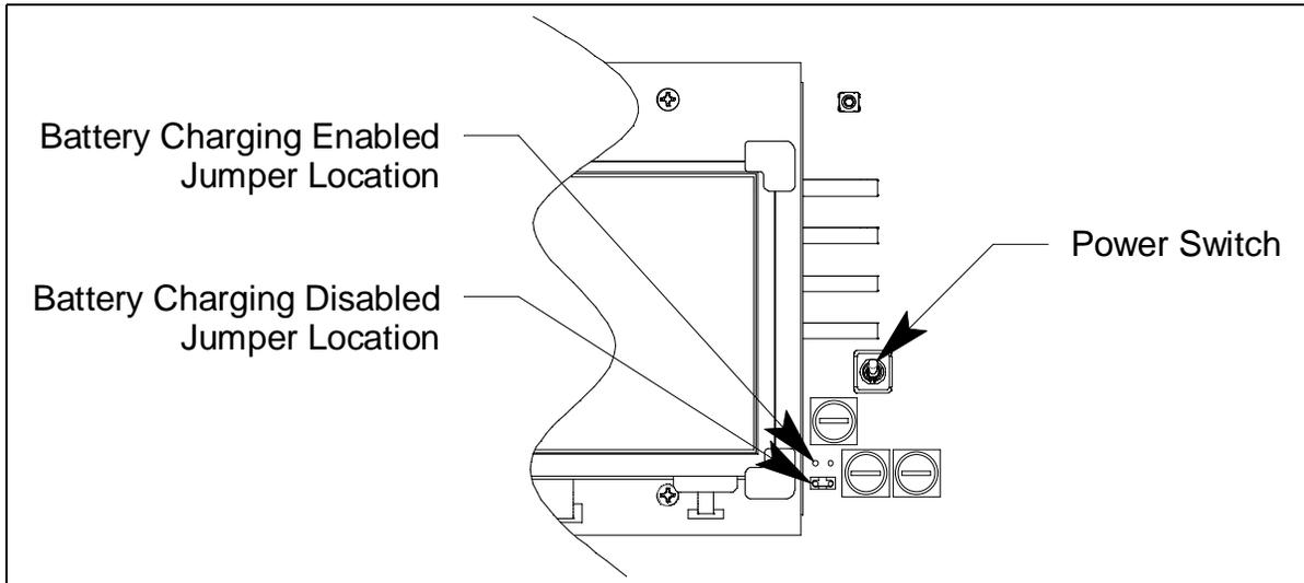
**Figure 38: Battery Charging Jumper Locations**
