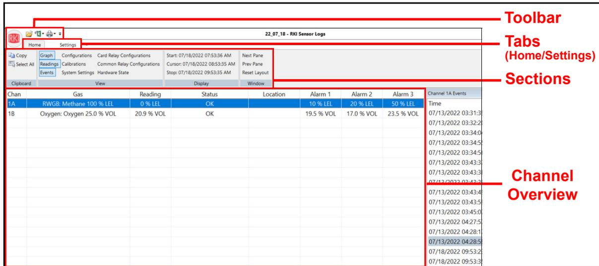
**Figure 129: Sensor Logs Program Interface**
