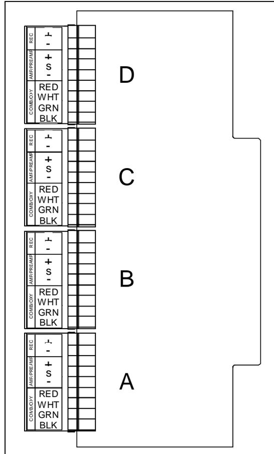
**Figure 28: Sensor Module Channel Assignment**
