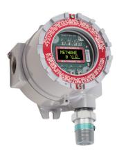
The M2A model is an explosion proof transmitter that can operate as a standalone system or as part of a system connected with an analog or digital signal to a controller, PLC, or DCS. The M2A utilizes a magnetic wand technique for performing non-intrusive calibration. The housing does not need to be opened for zeroing or calibration.
