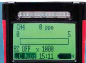
PPM Leak Check Mode
