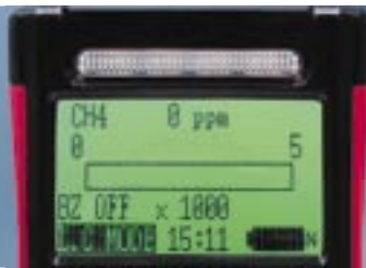
PPM Leak Check Mode
