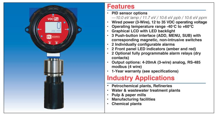
The VOC Pro Series Gas Detector is a versatile assembly that uses a PID sensor to detect a variety of gases. Wired power (12 to 35 VDC) with 4-20 mA analog and RS-485 Modbus outputs are standard. Magnetic switches allow for non-intrusive calibration while in the field as well as full system settings and diagnostics.
