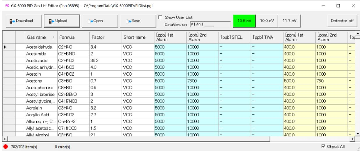
6. There are separate gas lists for the low/high range 10.6 eV sensors, the 10.0 eV/benzene sensor, and the 11.7 eV sensor.
