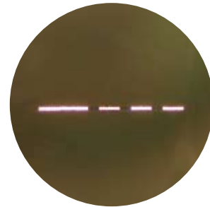
Array, 50 \mu m core fibers; Stripped buffer; Very short (150 mm)
